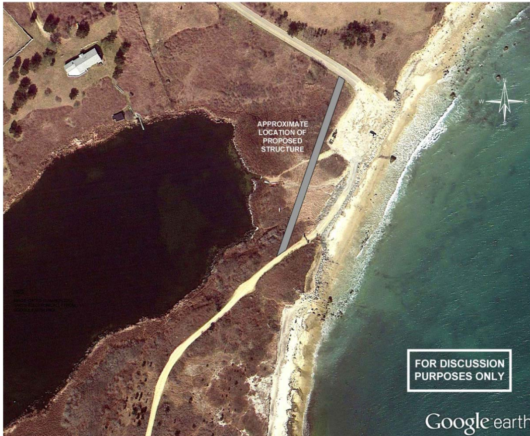
Figure 12. Proposed alignment of Elevated Roadway.
